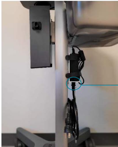
Power supply block and power supply cable connection
