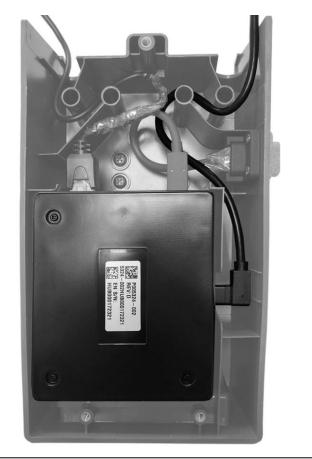
4 Connect the HUB Power supply DC cable (routed through the mouse hole).
