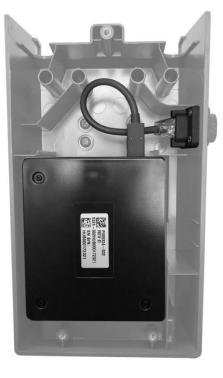
5 Route the USB cable to the right side and the power supply to the left. Route the USB cable up the column.
