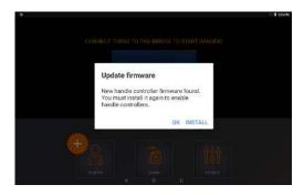
Press the INSTALL button on the popup to update the Handle Controller firmware and Kosmos Bridge will proceed to install the firmware.
