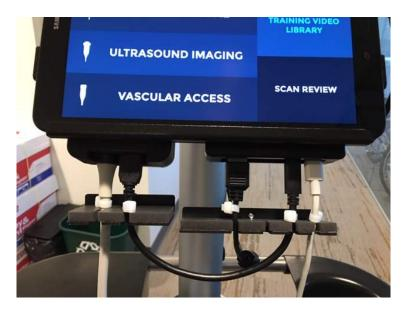
Additionally, the probe and power supply cable may be secured using a cable tie to the Bracket. See the picture below.
