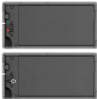
Figure 9. Securing the Kosmos Tablet G1 Batteries
