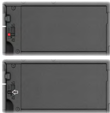
Figure 9. Securing the Kosmos Tablet G1 Batteries
