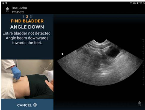
**FIGURE 18. Transducer positioning**
