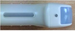
**FIGURE 17. Probe orientation marker**
