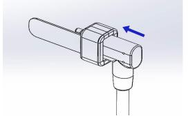
Plug the probe cable/connector combo into the tablet USB-C port but do NOT allow the adhesive to contact the tablet until Step 5.
